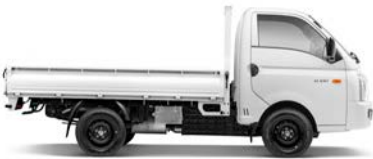
1 235 mm , Wheel base 2 430 mm , 1 185 mm , Overall length 4 850 mm
